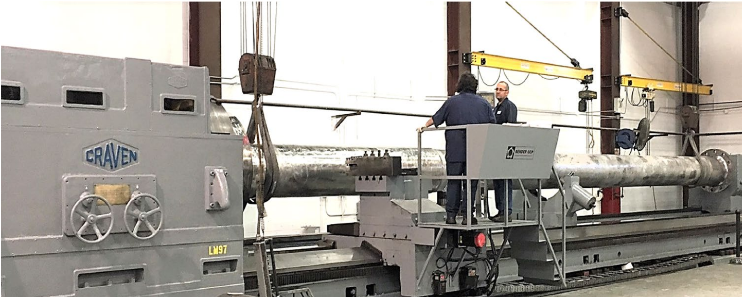
Bender CCP has several lathes dedicated to the manufacturing, repair, and overhaul of propulsion shafting, ranging in capacity up to 130 tons and 84 feet between centers.
