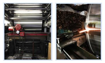
**Our Onsite CI Cylinder Restoration mobile units deploy quickly** for emergency repairs, or can be scheduled for planned downtime repairs and upgrades. Our highly skilled field service technicians are also FAA and Navy certified for the application of thermal spray coatings.
